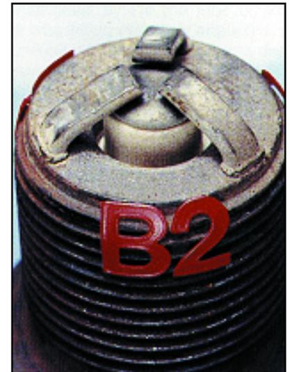
This plug was returned to us as one of a set of 12 that had operated for approximately 4000 hours in the fuel cells (pre-combustion chambers) of a turbocharged, four-stroke cycle, stratified charge, natural gas-fueled, stationary, V-angle, slow speed, 12-cylinder, integral compressor engine.
